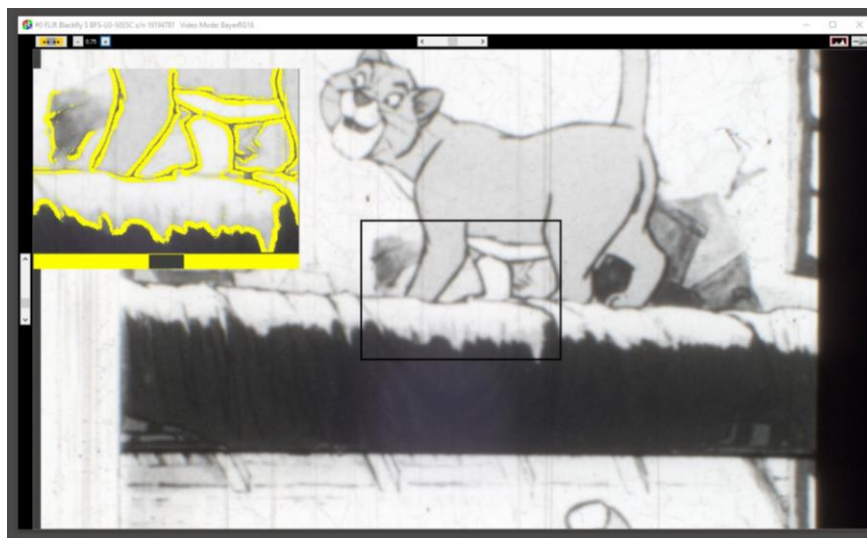
Focus aid mode activated by the Focus aid button
